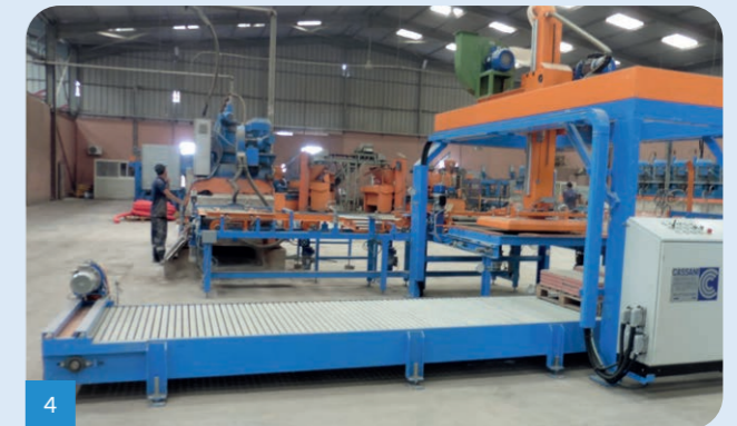
Motorised pallet loading/unloading bay.
