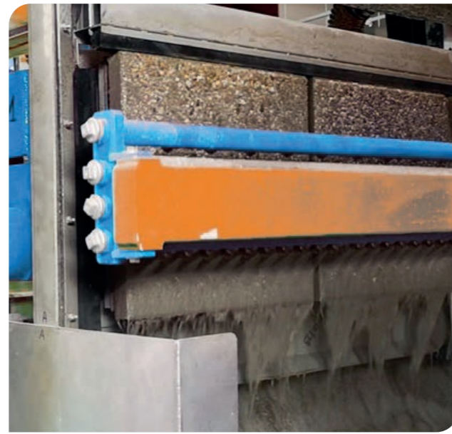
Wash-beton effect from direct washing process.
