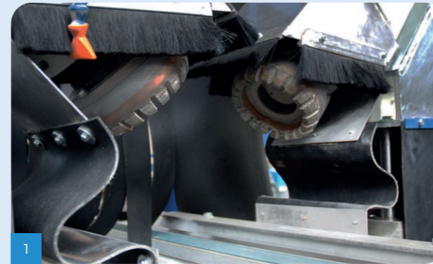
Details of chamfering heads at 45°.
