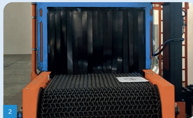
2 Entrance bay with metal mesh belt.
