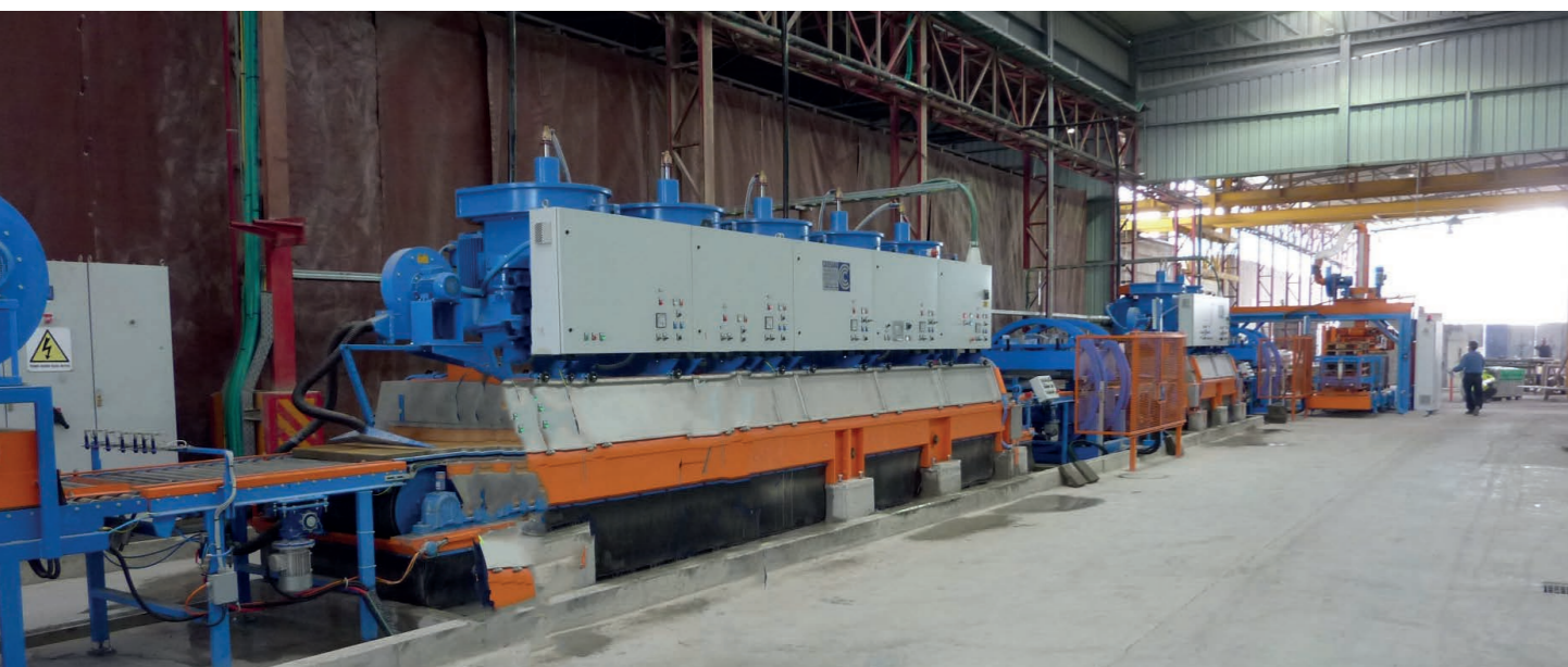
Calibrator, tilter and grinder in a plant (slabs are depalletized on the right and travel towards the left here)
