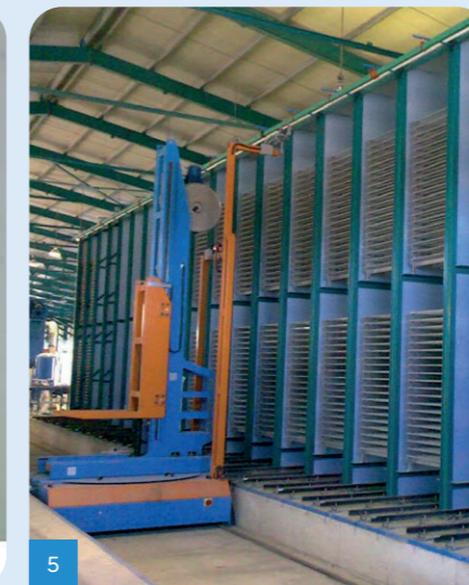
Robot trolley feeding curing chambers.
