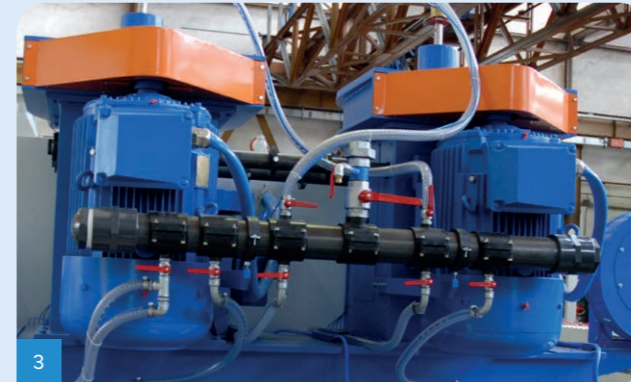
Cooling water distribution.
