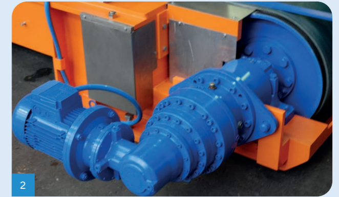
2 Belt conveyor moto-reductor.
