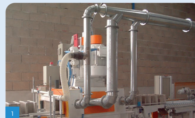
M 50 DRY / 1 Head, dust aspiration detail.
