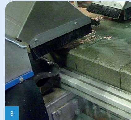
Chamfering of slabs.
