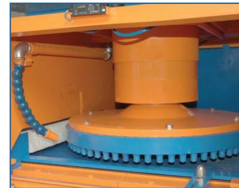
Station with vertical axe spindle with speed suitable to diamond abrasives in ring shape. With such a system , the diamond disk is positioned for working at wished level and the same ring does work locked in chosen position: from time to time, the level is corrected as to recover the tool weariness which in a short time is, by the way, non significant.
