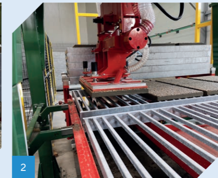
Horizontal depositing on trays.
