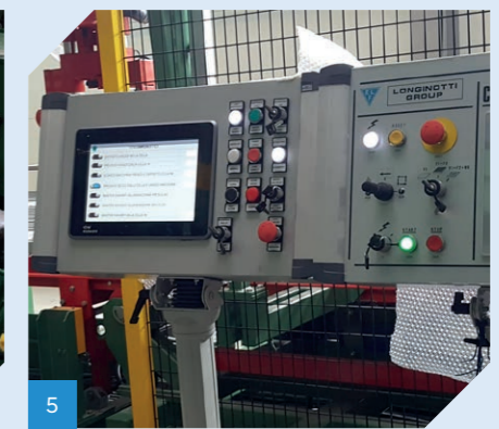
Integrated touch-screen control system
