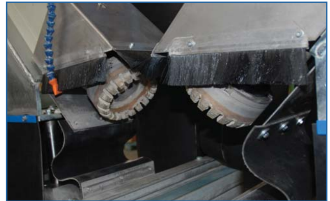
Details of chamfering heads at 45°
